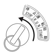
Figure 20. Key Switch (Stop)
